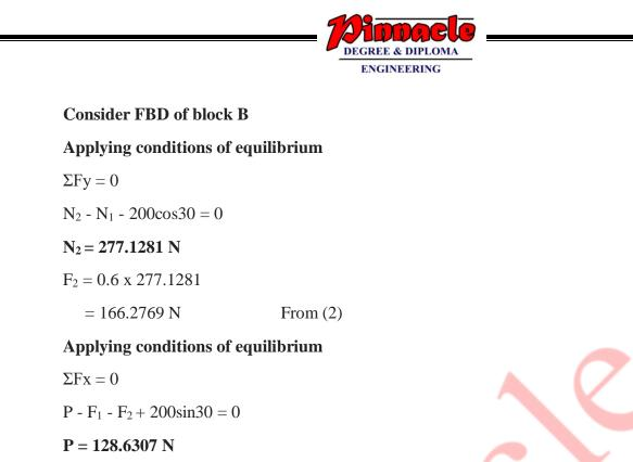
Force required on block B to start the motion is 128.6307 N
